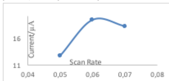
Figure 5. Calibration curve of the electrode scan rate (Sodium acetat buffer, pH 6.0; 50 mM, T, 40 °C).
